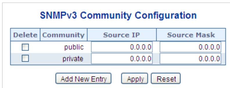
Figure 4-2-2-5: SNMPv3 Communities Configuration Page Screenshot
