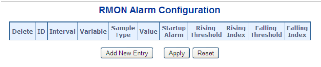
Figure 4-2-3-1: RMON Alarm Configuration Page Screenshot
