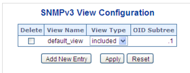
Figure 4-2-2-8: SNMPv3 Views Configuration Page Screenshot
