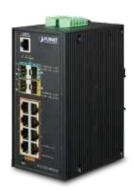
802.3at PoE+ & 10G Uplink DIN-rail Solution for Harsh Industrial Environment PLANET IGS-5225-8P2S2X is the smallest 10G uplink managed PoE switch in the industrial networking industry. Based on its 10Gbps big pipe connectivity to core networks, the IGS-5225-8P2S2X, equipped with 8 Gigabit ports featuring 36-watt 802.3at PoE+ and two 10Gbps SFP+ uplink slots, meets the demands of high power consumption and high bandwidth for 11ac Gigabit Wi-Fi APs, other PoE applications or
